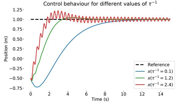
Fig. 2: Control behaviour for different values of  $\tau^{-1}$ . Higher values of  $\tau^{-1}$  potentially introduce overshoot oscillations.
