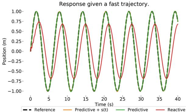
Fig. 5: Response given a fast trajectory  $\mu_d = \sin(t)$ .
